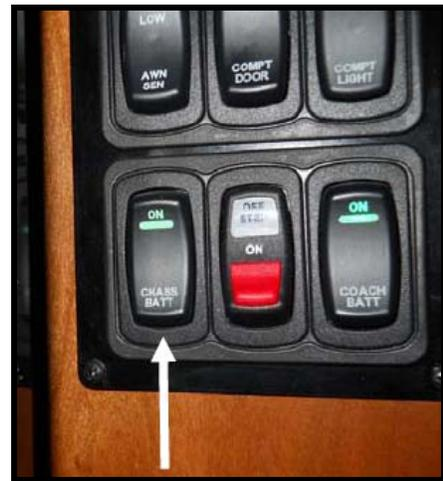
Figure 2 – Winnebago Industries Chassis Battery Disconnect Switch
